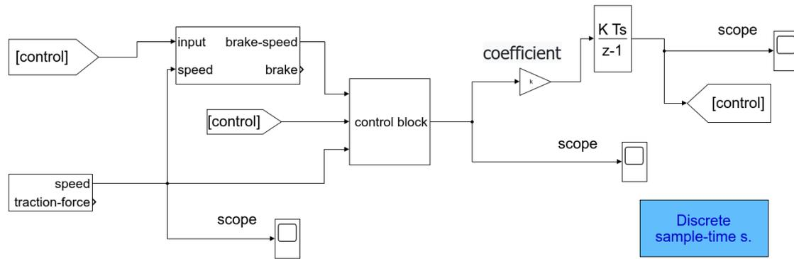
Figure 4. Simulation screen
