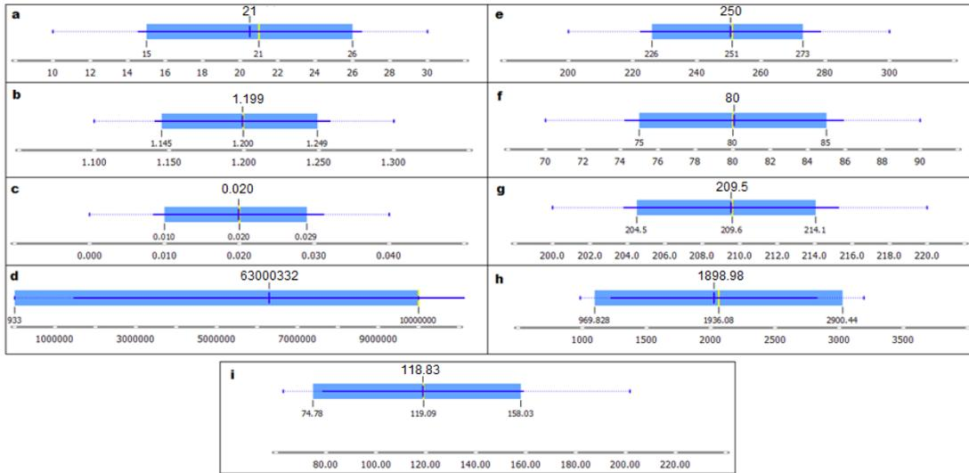
Figure 3. Distribution of input and output parameters that form the model. Input parameters: (a) Waiting Time (b) Motion Resistance, (c) Slope, (d) Curve, (e) Traction Force, (f) Maximum Speed, (g) Vehicle Mass, and (h) Distance Between Two Stations. Output parameter: (i) Travel time.
