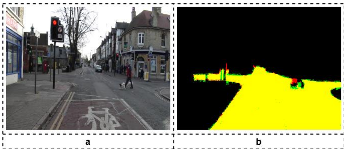
Figure 5 Visual results from the pedestrian detection system
