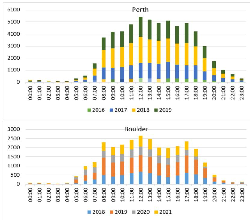
Figure 1 Charging start times of EVs for the Perth and Boulder datasets
