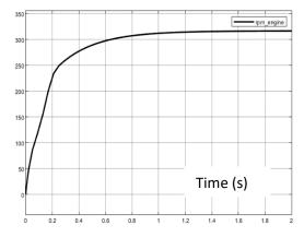
Figure 5. Diesel engine cranking rpm in normal behaviour
