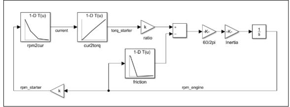
Figure 4. Diesel engine cranking model
