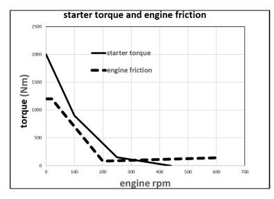
Figure 3. Starter torque and engine friction curves
