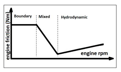
Figure 2. Stribeck Engine Friction Curve
