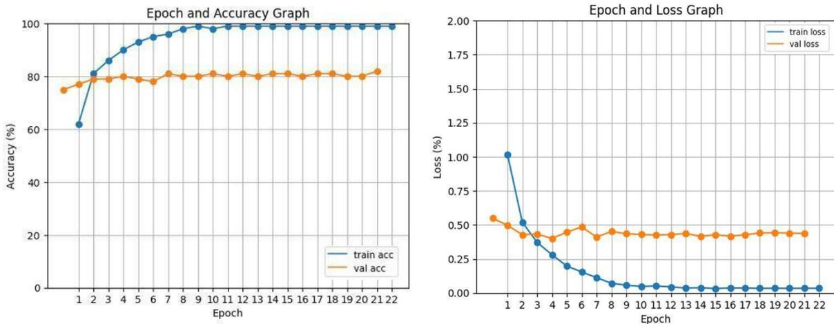
Figure 4. Accuracy and loss graph of MobileNetV2
