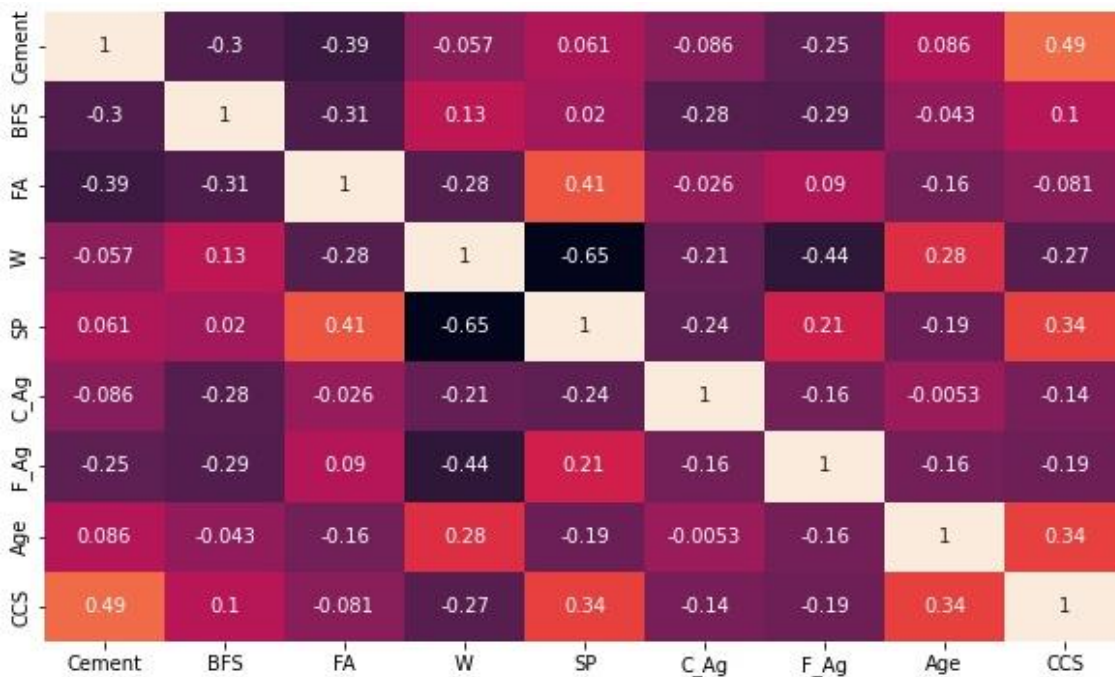
Figure 2. Pearson’s Correlation Plot of the Input and Target Variables
