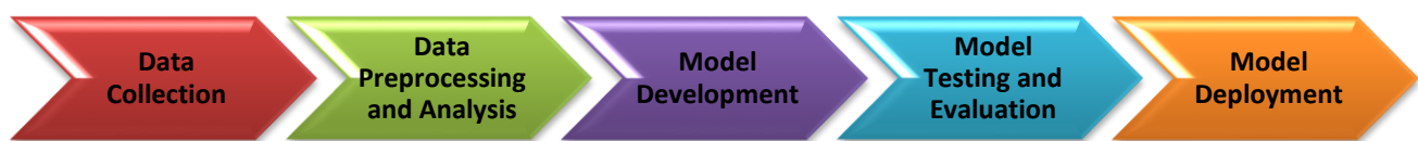
Figure 1. Concrete Compressive Strength Prediction Process Flow Diagram
