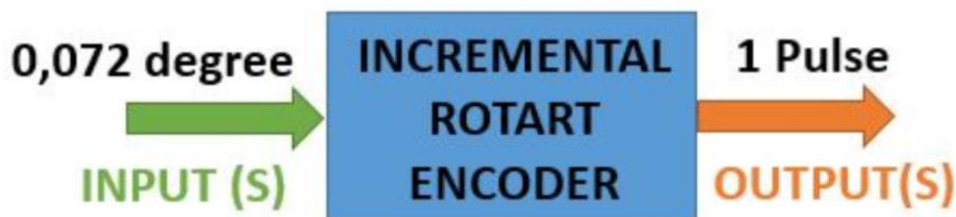
Figure 11. Incremental Rotary Encoder Block Diagram
