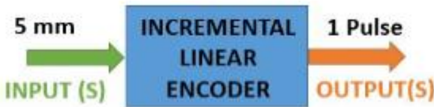
Figure 13. Incremental Linear Encoder Block Diagram
