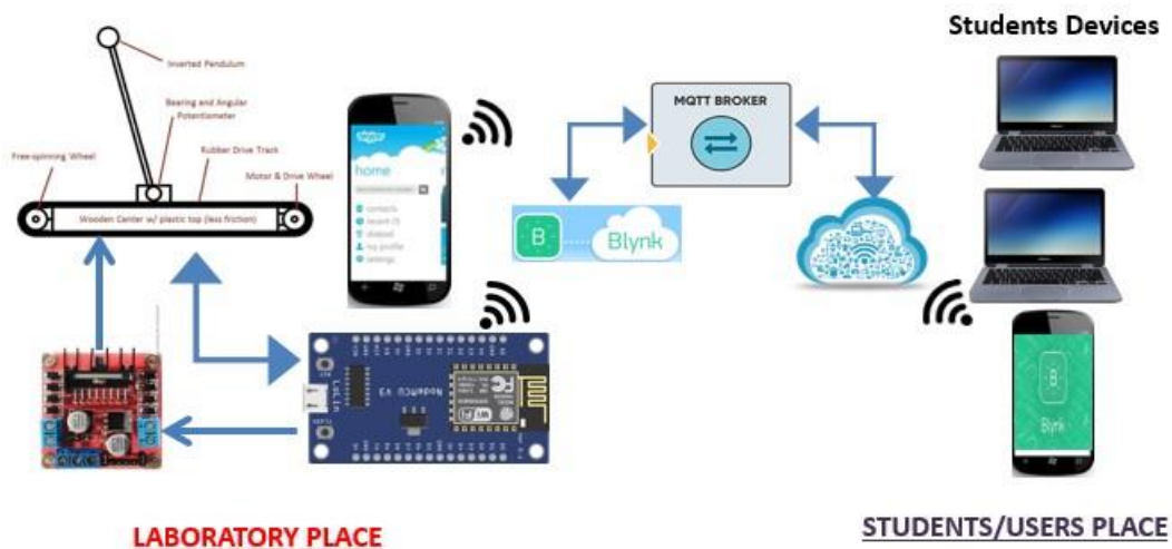
Figure 20. Schematic of the Developed Lab Experiment System
