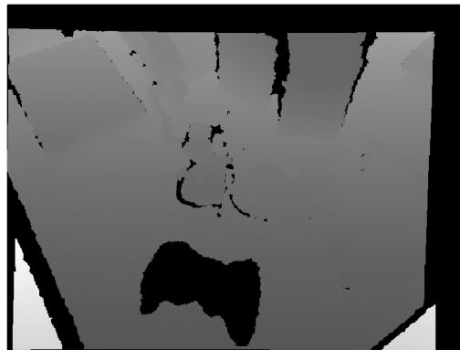
Figure 2: Distortions on the Edges of the Joystick Object in the Depth Image
