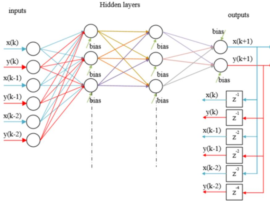
FIGURE 8. Nonlinear Autoregressive Neural Network (NAR) Structure
