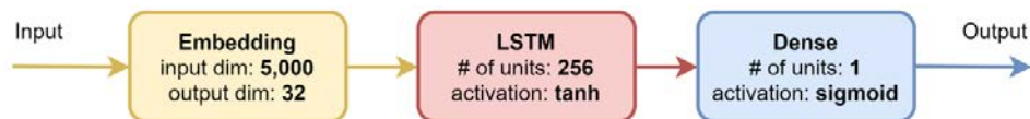
Figure 6 A block representation of the architecture of the proposed sample LSTM model
