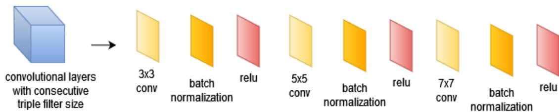
Figure 2 The structure of convolutional layers with CTFS
