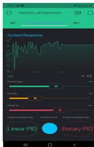
Figure 8. GUI Showing the Time-Response of Inverted Pendulum and PID Controller Values on the Blynk Platform
