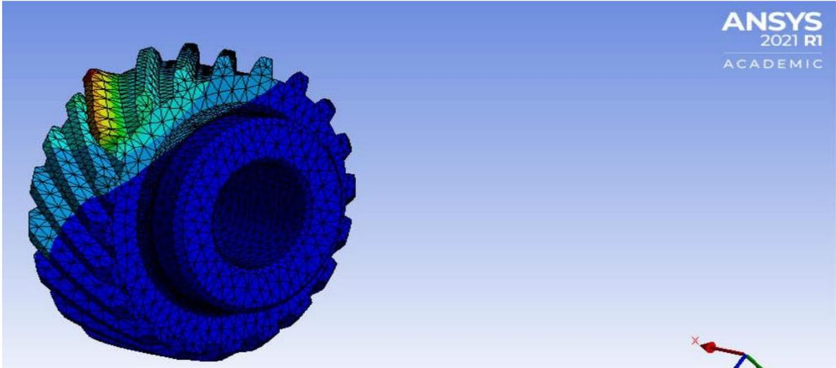
**Figure 8.** Deformations in helical gear wheels.
