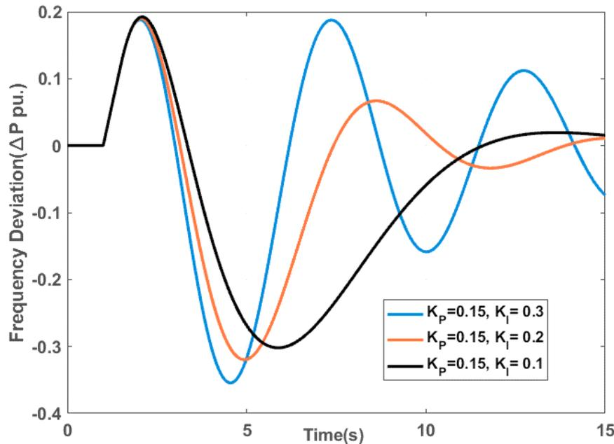
**Figure 5.** Frequency deviation for different controller gains ( $\tau = 0.5$ sec)
