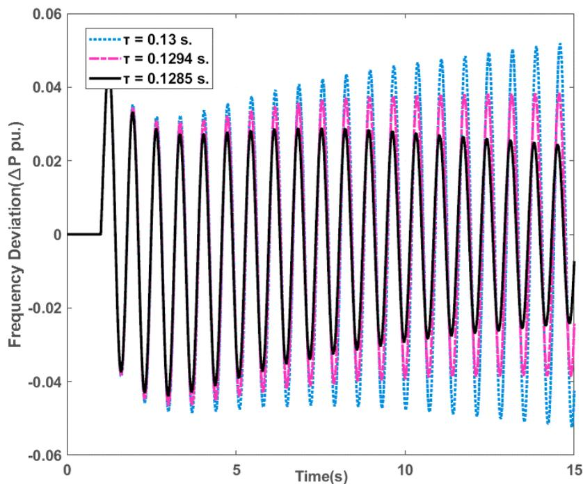
**Figure 4.** Frequency deviation for different time delays ( $K_I=3.5$ ,  $K_P=3$ ,  $\tau^*=0.1287$ )
