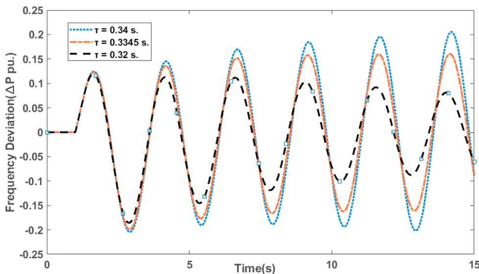
**Figure 3.** Deviation of load frequency versus time delays ( $K_I=1, K_P= 0.5, \tau^*=0.3345$ )
