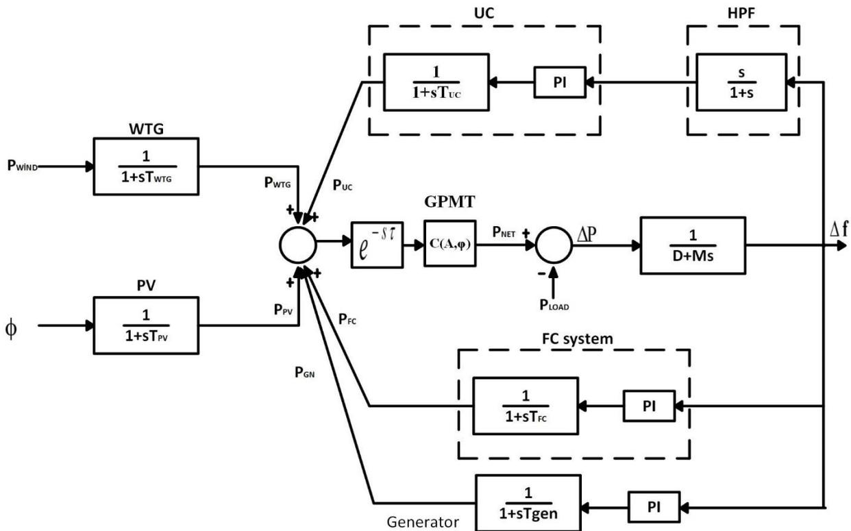
**Figure 2.** Hybrid power system block diagram for investigation.
