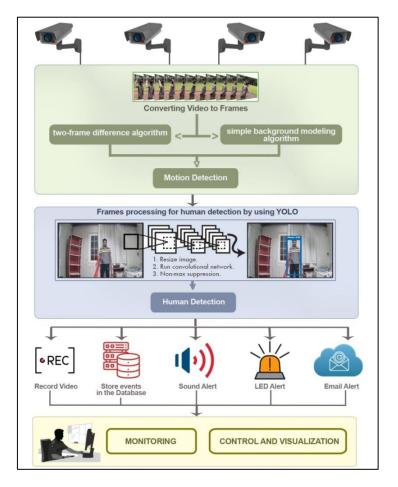
Figure 5: Architecture of the security alert system
