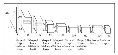
Figure 3: Tiny YOLOv2 Architecture [22]
