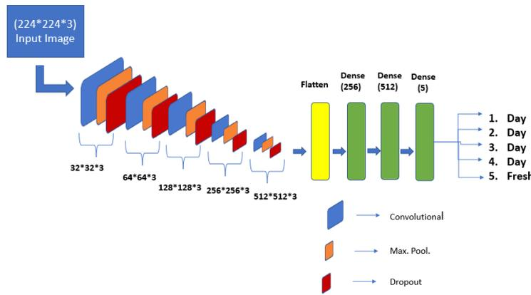
Figure 3. The designed CNN model architectural structure
