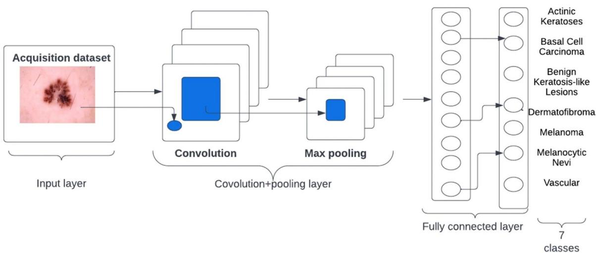
Figure 1 Overview of CNN Architecture [13]
