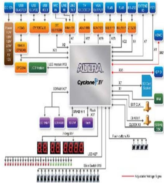
Fig. 10. Block Diagram of DE2\_115 FPGA Board.
