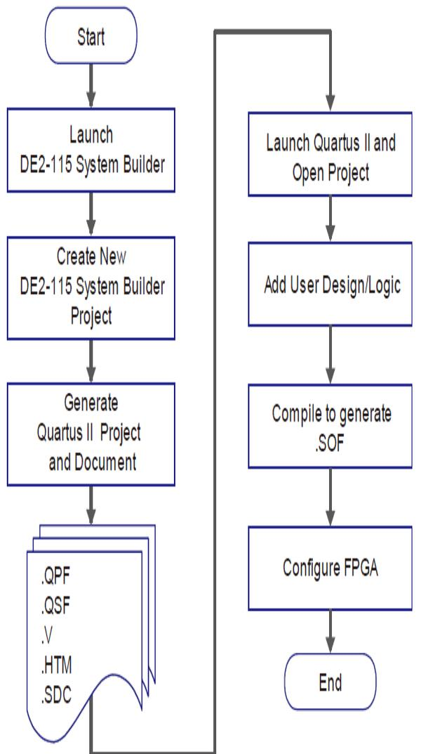
**Fig. 11.** The flow chart of the software carried out in the Quartus program
