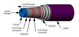
Figure 3 The Cold dielectric (CD) superconducting cable design
