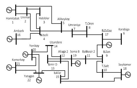
Figure 2 The Turkish 22 Bus 380kV transmission system
